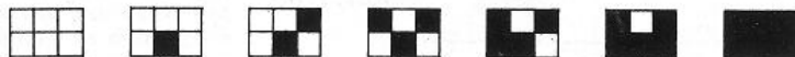
Figure 5: Grey-level rendition on the Sirius screen. Each image pixel uses 3 x 2 screen pixels; grey levels are simulated by changing the number of lit screen pixels within the 3 x 2 block.
