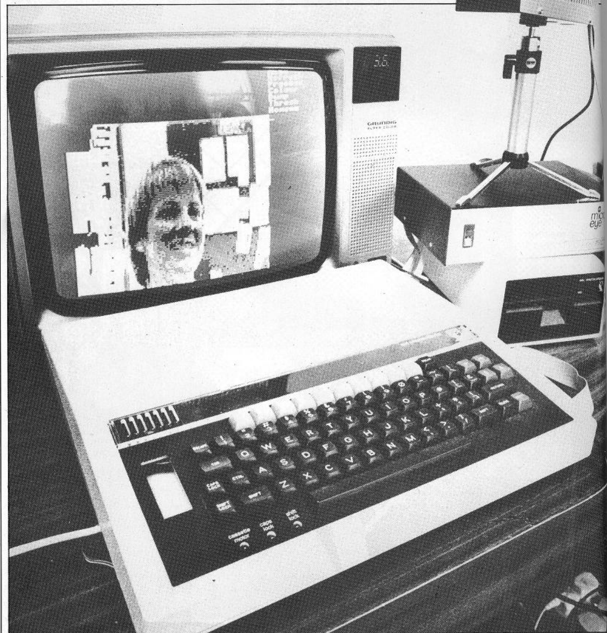
The complete system: closed-circuit TV camera, Microeye interface and BBC micro — plus a digitised PCW Editor!
